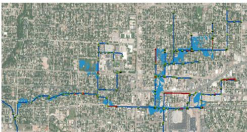
Subsurface drainage modelling using Flood Modeller-SWMM in Colorado, USA
