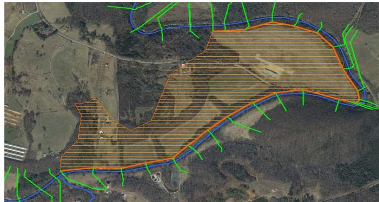
Stream modelling and mapping within the Etowah Basin and Bannister Creek was compared with the Flood Modeller Pro results. Since the initial models were 1D, initial comparisons were performed in 1D. Later review of the models identified areas where 2D modelling might be used to better represent shallow overland flow.
