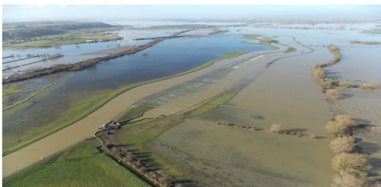
Transfer of flow between river systems over Allermoor spillway
