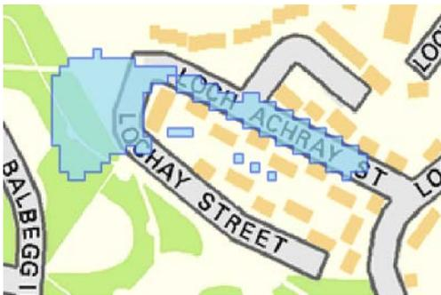
The above image shows a street in Glasgow where predicted pluvial flooding shows good agreement with the post event flood report data (which identified Loch Achray Street as having been subjected to extensive internal and external flooding).
