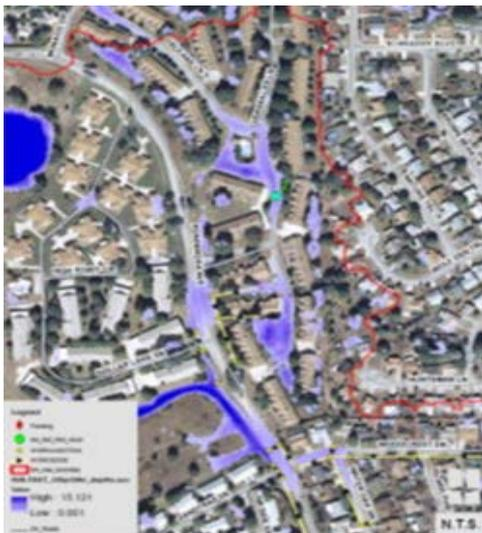
To help deliver an accurate, terrain based watershed evaluation, multiple topographic data sets from a variety of sources were edited. An extensive review to identify data gaps and assess the available data for breakline issues (e.g. missing or raised breaklines), filtering issues (e.g. vegetation remaining within the surface), and tie edge effects was also performed.
