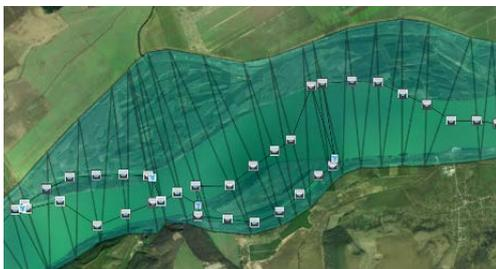
*Flood Modeller TIN of the Popina critical location in the lower Danube and 1D model network*
